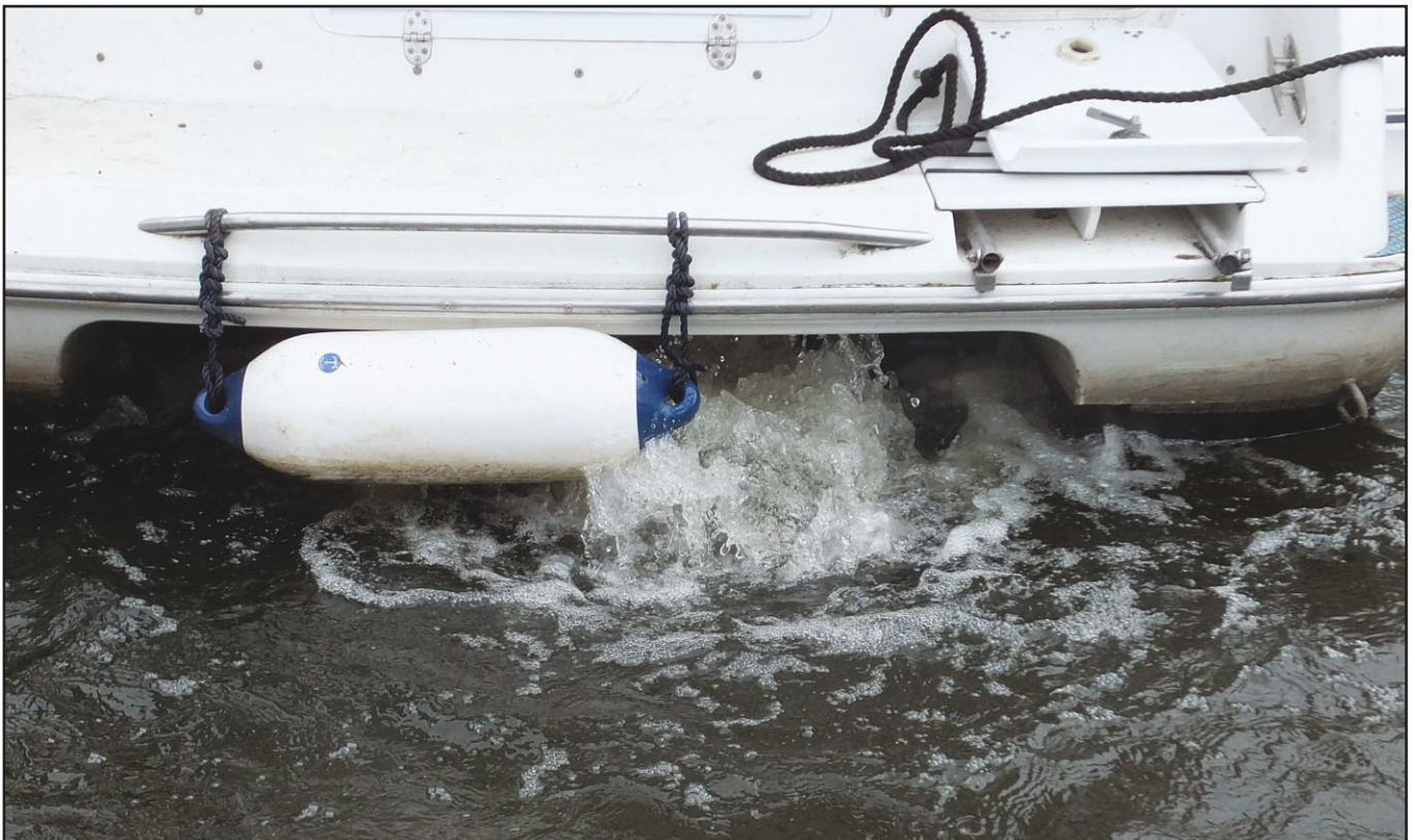
Figure 2: Wet exhaust at boat's stern
