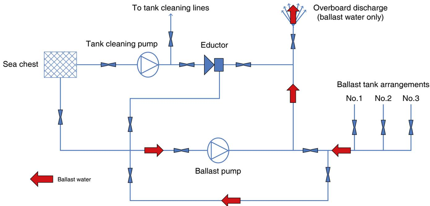
Diagram 1 – Simplified ballast system – deballasting with main ballast pump
