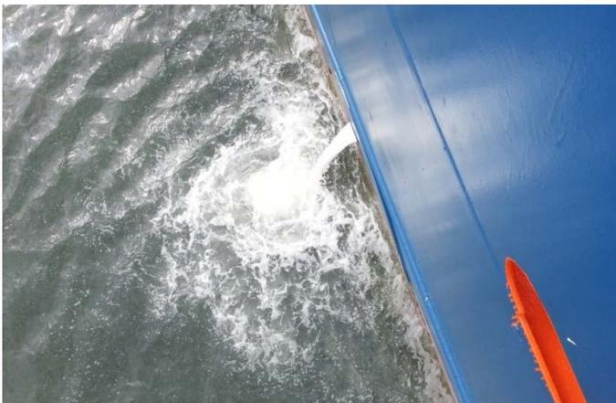
Figure 7 – Overboard discharge of eductor when running on local harbor water with ballast tank lines closed – an aerated plume of comparatively clean water – courtesy Douglas Smith
