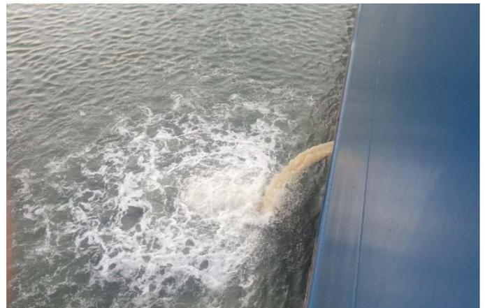
Figure 8 – The same discharge water when the eductor is connected to a ballast tank - the discharge is now both aerated and discolored by sediments in the connected ballast tank – courtesy Douglas Smith
