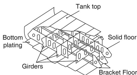
Figure 1 – Typical double bottom ballast tank construction
