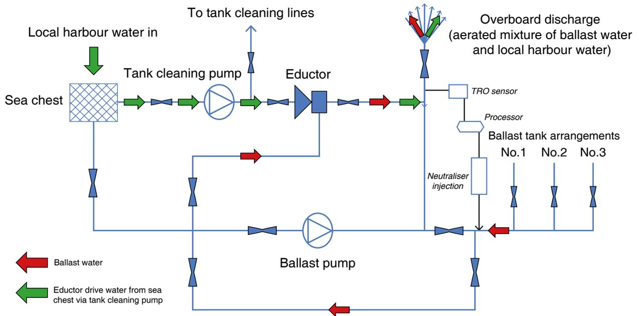
Diagram 3 – Simplified ballast system – deballasting (stripping) with eductor and neutraliser injection
