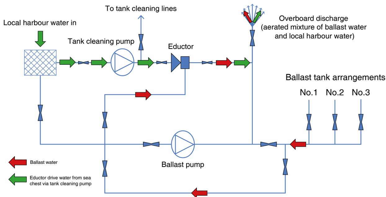
Diagram 2 – Simplified ballast system – deballasting (stripping) with eductor
