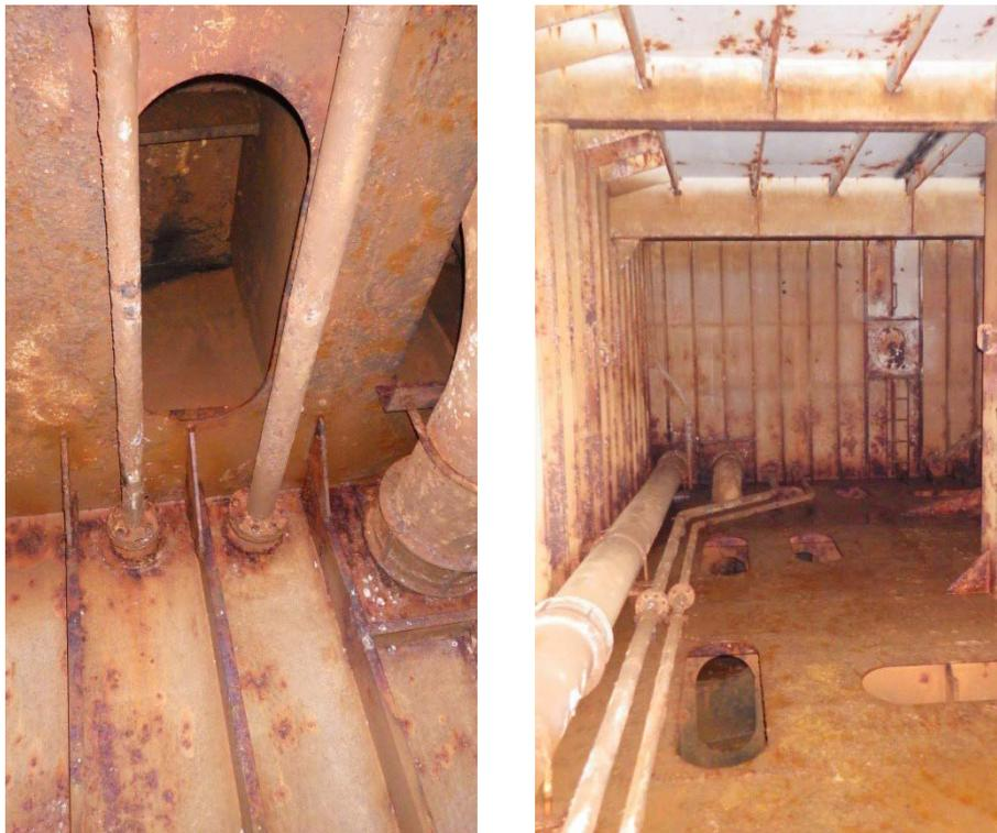
Figure 5 – Illustration of poor internal ballast tank condition – rust and scale deposits can also lead to the blocking of designed draining arrangements.
