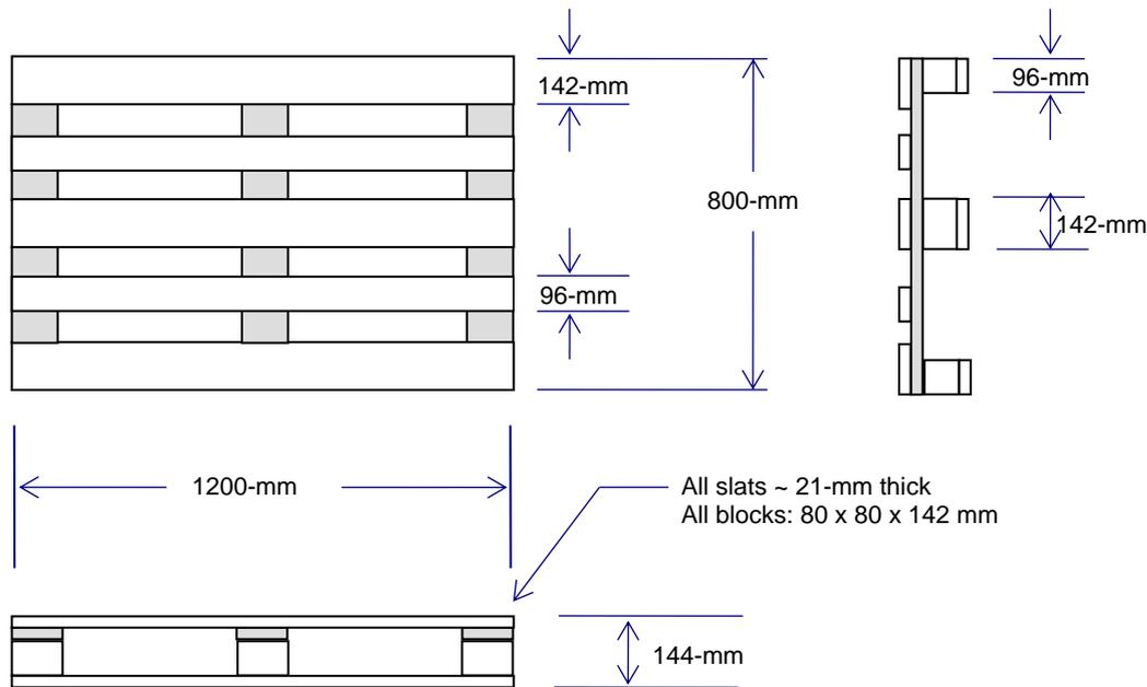
**Figure 3.2.1 – Typical dimensions of the standard EUR pallet**
