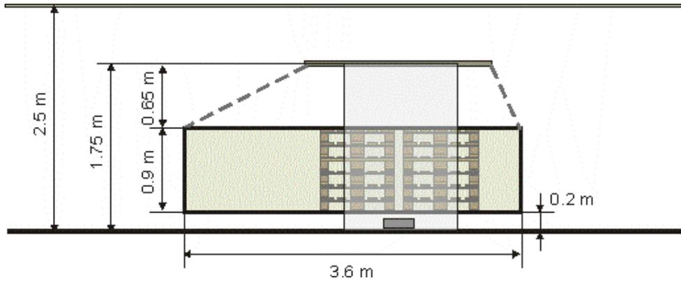
**Figure 3.3.3.1 – Side view of the passenger vehicle fuel package**
