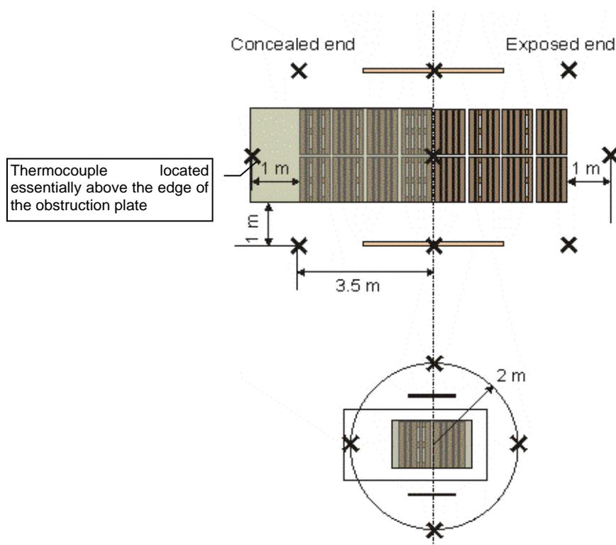
Figure 3.5.1 – Thermocouple locations in the two scenarios<sup>3</sup>
