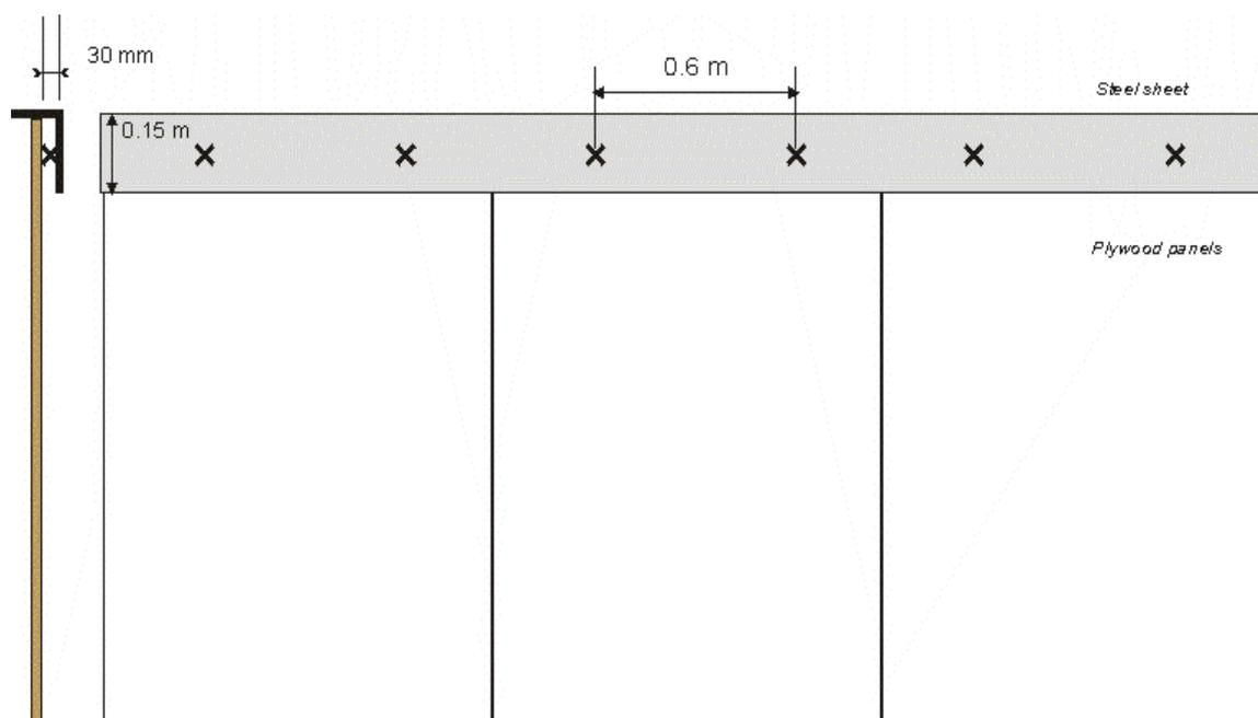
**Figure 3.5.2 – Thermocouple locations at the plywood targets for determining ignition of targets<sup>4</sup>**
