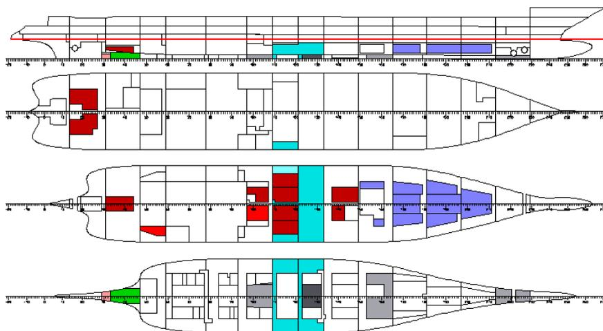
Fig. 3: Example of damage stability assessment based on an actual loading condition
