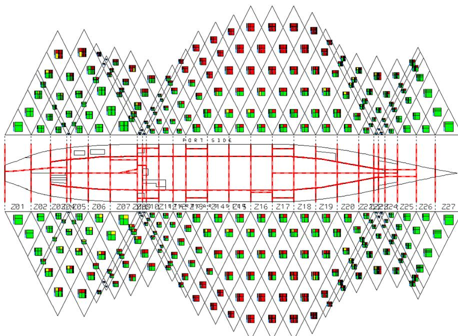
**Fig. 2: Examples of survivability indexes computed for a ro-ro vessel taking into account multiple-zone damage at max. draught. Severity of damage reported on a “color-based” scale.**
