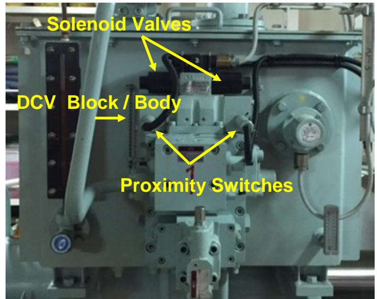
Ignoring the problem meant that although the rudder moved as expected in these two cases, the lack of properly functioning proximity switches might result in a failure to detect if the rudder had not moved, since crewmembers had trained themselves to ignore the alarm.
