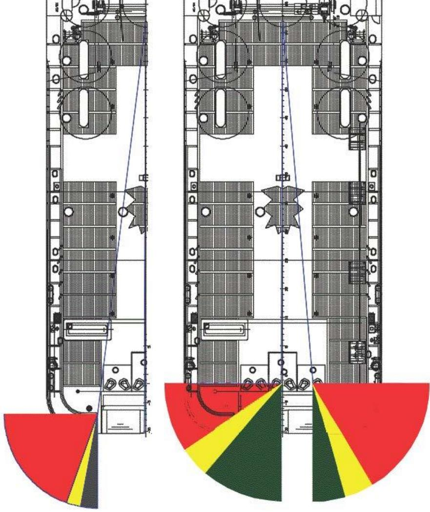
Figure A3-2: Illustration of the operational, cautionary, and stop work zones (coded respectively "Green", "Yellow" and "Red" zones)
