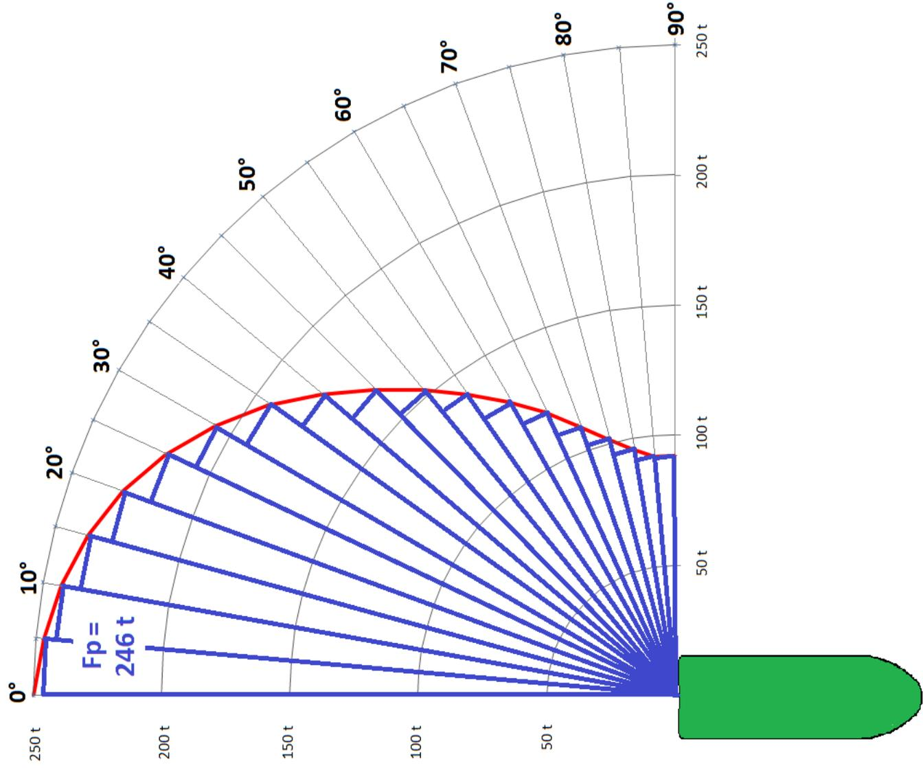
Figure A3-3: Permissible tension sector diagram based on standard alpha values
